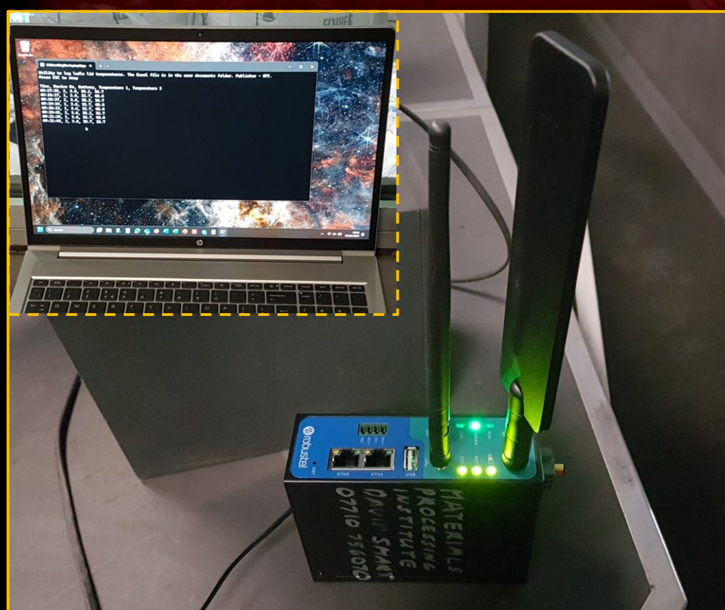
Figure 4: LoRaWAN gateway receiving signal data from lid transmitters. Inset Image: Initial data being received on a laptop.
