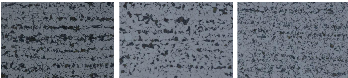
100 μm Samples isothermally transformed at (a) 700 °C (b) 650 °C (c) 600 °C
