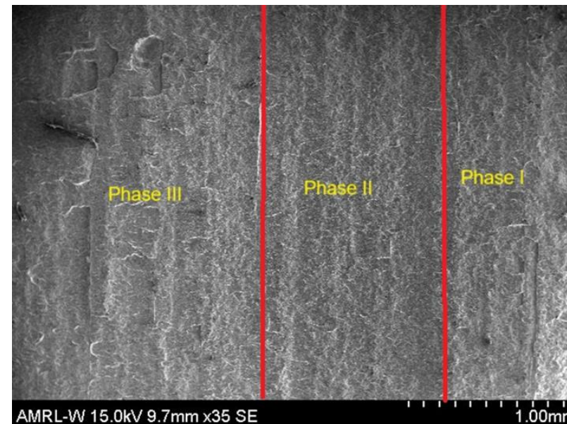
Fig 14: SEM images of the fractured CT samples
