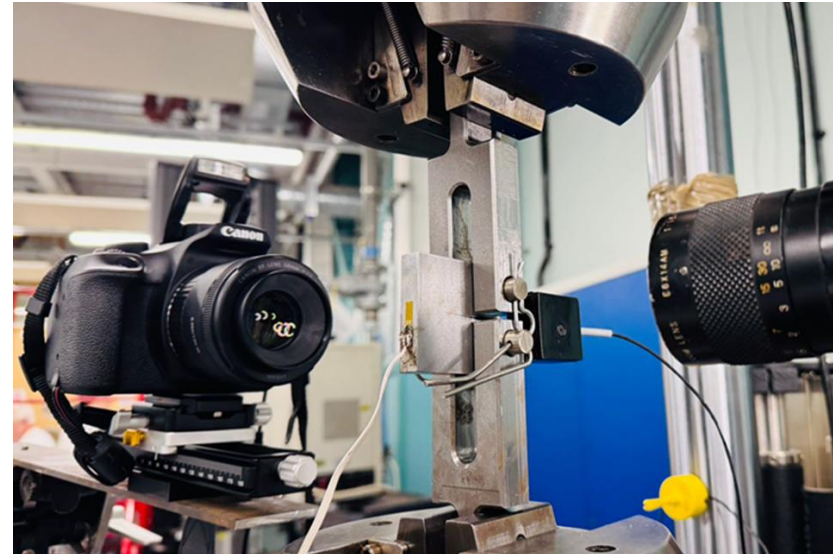
Fig 12: Visual crack monitoring technique
