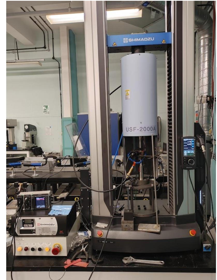
Fig 6: UFT test setup at the lab
